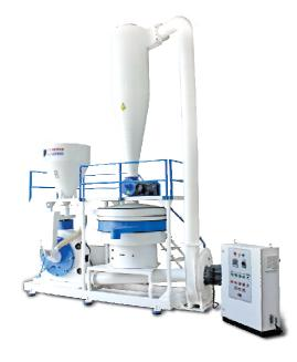
PULVERIZERs are used in application like pulverizing of Rigid & Soft PVC, uPVC and cPVC scrap waste in PVC processing industry & pulverizing HDPE, LDPE, LLDPE and various other thermoplastic materials for Rotational-Molding, compounding and master-batching applications where material are required in fine powder form.
