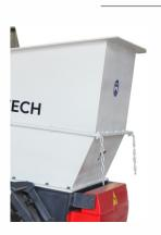
The hopper fulfils several tasks at once. First, the material to be shredded is fed through it – manually, mechanically, or by conveyor belt. The generous opening makes it easy to fill even very large parts. A decisive factor for shredding, however, is its special design, which is rounded at the front and thus effectively prevents material bridging. Even with bulky parts, the shredder cuts itself free. If required, hopper extensions and lids with gas pressure springs are available.
